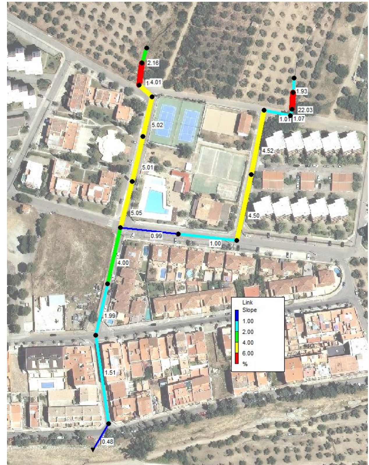
Pendents longitudinals conductes
